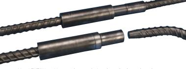
nVent LENTON position couplers are designed to splice bars where the ongoing bar is restricted in its axial movement or cannot be rotated and length adjustability of the coupler is required.
