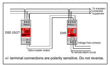
When connecting the DAR to multiple opto-couplers the opto-couplers should be connected in series with + terminal of one connected to the – terminal of the next. The DAR + terminal should connect to + SPD terminal at one end of the series connection and the – DAR terminal connect to the – SPD terminal at the other end of the series connection.
