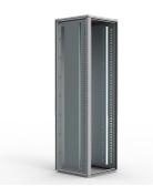
The galvanised steel internal side panels, MSPS, segregate vertical sections and allow for mounting of busbar supports, MHSH, as well as other accessories. It is a flexible solution both for fix and plug in systems and allows for meeting form 4 segregation according to IEC 61439.
