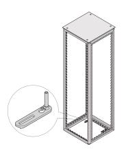
Tip-Over Protection helps make floor mounted enclosures stable and prevents tip overs due to load imballance. The tip over protector can be assembled on the frame or the plinth.
