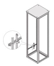
For cable ducting in side area of cabinet.
