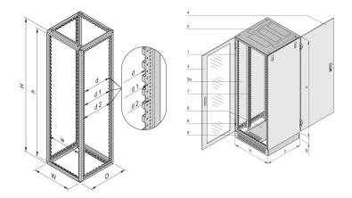
Basic rack to support cabling and networking equipment. Cooling via convection or top cover fans.
