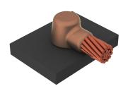
nVent ERICO Cadweld Cathodic Connections are the preferred method of exothermically welding cathodic protection anode leads to pipes (steel or cast iron), tanks, and other structures. Cathodic protection systems are designed to prevent galvanic corrosion along a pipeline or in various structures. nVent ERICO Cadweld Cathodic Connections use a special welding material alloy to minimize heat effect on the steel, which is especially important on thin wall and high stress pipes.
