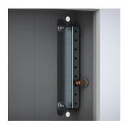
These mounting profiles can be fitted into the terminal box to allow for DIN rails to be easily installed, exactly where required, for the mounting of modular components, eliminating the need for using the box's mounting plate.
