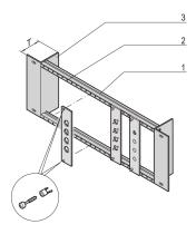
Module support is needed for assembly of partial width front panels with SUB-D-, ST type 3 or FDDI cut-outs, with or without strain relief rail.
