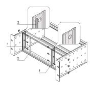
For vertical textile EMC shielding between recessed mounted shielded front panels and side panel.
