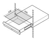
Writing surface to use with our 19" drawer. It is placed on the drawer and I can be lifted up when the drawer is open.
