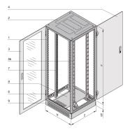
Basic rack to support cabling and networking equipment. Cooling via convection or top cover fans.
