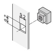
Square nuts have higher contact surface and dont get rounded off unlike hex nuts. For precise, anti-twist secure mounting without clearance, use square nuts.
