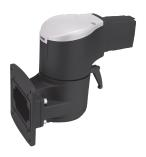
Syspend 180-Max Horizontal Panel Coupling mounts a horizontal tube to the back of an enclosure or screen using Video Electronics Standards Association (VESA) mounting. The coupling has mounting holes drilled for standard VESA 75 and 100 flange sizes. It enables the enclosure to rotate 300 degrees and can be locked into a given position. The horizontal panel coupling has a safety stop and maintenance-free bearings.
