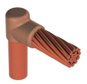
nVent ERICO Cadweld Cathodic Connections are the preferred method of exothermically welding cathodic protection anode leads to pipes (steel or cast iron), tanks, and other structures. Cathodic protection systems are designed to prevent galvanic corrosion along a pipeline or in various structures. nVent ERICO Cadweld Cathodic Connections use a special welding material alloy to minimize heat effect on the steel, which is especially important on thin wall and high stress pipes.
