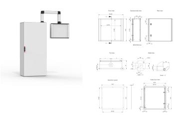
The mild steel operator interface control enclosure, OICE, has a pre-machined hole pattern to allow for the fixation to a swing arm, plus a removable front plate at an IP 55 protection degree. Components can be easily fitted thanks to the removable front plate, but will also be easily accessible through a rear door. Side handles on the enclosure allow for easy movement of the enclosure into the working position.
