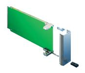
Handle mechanism AMC.0 Rev. 2.0, MTCA.1 and MTCA.4 Modules.
