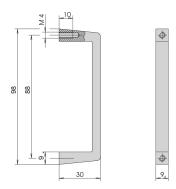
Slim Aluminium profile front handle, 9 mm. The assembly of the handle will be done from the rear side.
