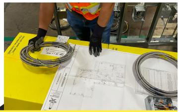
nVent CADDY CPS scales with projects by providing advanced prefabrication assemblies that are UL-listed, designed to strict specifications, and assembled in a controlled environment.
