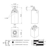
Switch for connecting to the normally closed contacts of the door control module for manual door opening. This primarily is used for lights and cooling solutions which should be linked to the opening or closing of the door.
