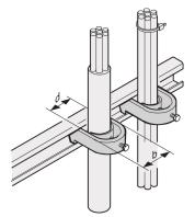
C-Rails are for better cable management. Installation generally behind the 19" uprights. They are compatible with standard cable clabs.
