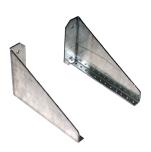
The Equipment Rack Angles can be added to 36-in. and 48-in. tall cabinets for extra 19-in rack equipment mounting. The EIA spaced holes are tapped 10-32. They mount to raised pads on the cabinet back on the inside with the hardware that is provided.
