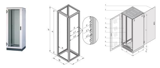
Basic rack to support cabling and networking equipment. Cooling via convection or top cover fans.
