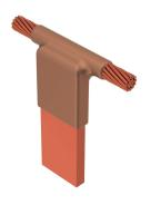
nVent ERICO Cadweld Cathodic Connections are the preferred method of exothermically welding cathodic protection anode leads to pipes (steel or cast iron), tanks, and other structures. Cathodic protection systems are designed to prevent galvanic corrosion along a pipeline or in various structures. nVent ERICO Cadweld Cathodic Connections use a special welding material alloy to minimize heat effect on the steel, which is especially important on thin wall and high stress pipes.
