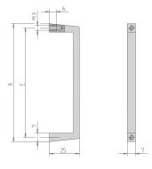
Slim Aluminium profile front handle, 7 mm. The assembly of the handle will be done from the rear side.
