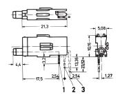
Test sockets for mounting plane 1 and 2, short and long type.
