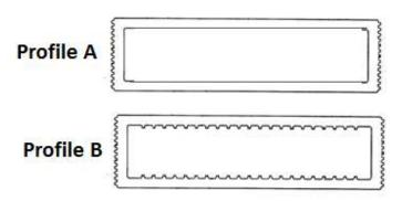
The insulating sleeve is compliant with Chapter 8.4.4 – Protection by total insulation of the IEC 61439-1 standard (Class II: reinforced/double insulation)
