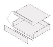
The EMC shielding kit and the cover plates increase the shielding of the chassis from approx. 30 dB(A) to approx. 60 dB(A). A test report can be downloaded.
