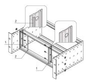
For vertical textile EMC shielding between recessed mounted shielded front panels and side panel.
