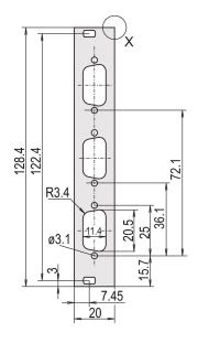
Flat front panel with cutout for D-Sub connectors. Unshielded version.
