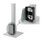
Syspend Vertical Motion Floorpost with Junction Box provides a method for mounting the Syspend VL and VHD Motion Arms when a structural surface is not available. It allows for a HMI enclosure attached to the Syspend VL and VHD Motion Arms to be post-mounted.
