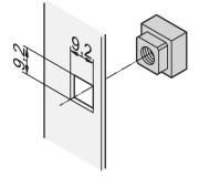
Square nuts have higher contact surface and dont get rounded off unlike hex nuts. For precise, anti-twist secure mounting without clearance, use square nuts.
