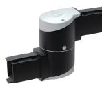
Syspend 281-Max Intermediate Joint to join two horizontal tubes together for a longer run. Arm can be rotated or turned 300 degrees. Includes safety stop and maintenance-free bearing. Use of the Intermediate Joint reduces the system load capacity to 179 lb. (81.2 kg) at 3.3 ft. (1 m).
