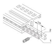
Perforated strip out of 1mm Aluminum for centering shielded plug-in units.
