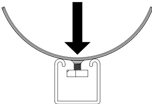
2. Rotate shield so it is positioned perpendicular to channel.
