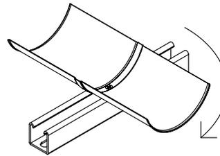
3. Rotate strut nut so it is positioned perpendicular to channel. Tighten strut nut so it seats with the channel flanges.
