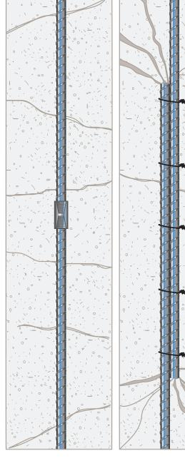
Mechanical splicing provides the assurance of maintaining load path continuity of the structural reinforcement independent of the condition or existence of the concrete Lap splices rely on bond with the concrete for effective continuity of reinforcement, which can result in localised areas of increased concrete stress that must be considered by the designer
