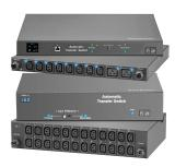
The Rack Automatic Transfer Switches provide power redundancy to rack-mount IT devices that are not designed to take advantage of data centers' second power source. The ATS devices provide power failover for single-corded devices.
