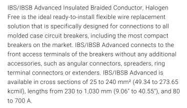
Manufactured in an ISO 9001 2015 certified automated facility, IBS/IBSB Advanced is formed by weaving high-quality electrolytic copper wire to form a durable low voltage connector with maximum flexibility which allows for more compact power connections to circuit breakers. The IBS/IBSB Advanced allows users to reduce the total size and weight of the installation, improving both design flexibility and assembly aesthetics.
