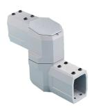
Compact Series 2 Intermediate Joint joins two horizontal tubes together for a longer length and creates a pivot. The arm can be rotated 360-degree with limit stop. Includes access plates for easy wire installation. Use of the intermediate joint reduces pendant arm load capacity by 43 percent.
