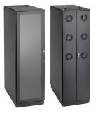
The ProLine FloTek FD Server Cabinet uses the cooling power of two banks of independently-powered fans in the back of the cabinet and an integral front floor duct to direct air into server intakes when positioned over a cutout in a raised data center floor. The cabinet air inlet requires alignment with a floor cutout so blocking plates can direct cool air from the floor plenum across the front of the equipment.
