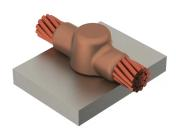
nVent ERICO Cadweld Cathodic Connections are the preferred method of exothermically welding cathodic protection anode leads to pipes (steel or cast iron), tanks, and other structures. Cathodic protection systems are designed to prevent galvanic corrosion along a pipeline or in various structures. nVent ERICO Cadweld Cathodic Connections use a special welding material alloy to minimize heat effect on the steel, which is especially important on thin wall and high stress pipes.
