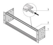
For mounting installation devices in accordance with DIN 43880 in sizes 1-3 with snap-in technology e.g. mounting sockets, circuit breakers or residual current circuit breaker. These can be fitted after the horizontal rail with lip DIN central rail (35/7.5) are fitted.
