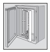
Swing Frame provides 19-inch rack-mounting capabilities with U-Style (Type RA) mounting hole pattern. Quarter-turn latch has 100-degree swing. Adjustable mounting provision. Swing frame maintains enclosure rating if properly installed in an nVent HOFFMAN enclosure. Front mounting position is approximately 140mm (5.5 inch) back on 400mm enclosures. Includes mounting hardware and instruction manual.
