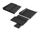
The Pivoting Keyboard Shelf pulls out and pivots 90 degrees to access full-size keyboard mounts either in a cabinet or on a 19-inch open-frame rack. The shelf allows a keyboard to slide between standard rack angles and includes a mouse tray. The keyboard tray extends 9.75 inch (248 mm) beyond the front of the rack angles or open-frame rack.
