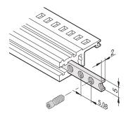
The threaded insert is a metal strip with thread M3 and allows the fixing of front panels.
