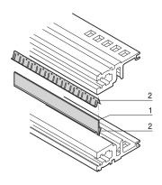
The contact strip makes contact bewteen horizontal rails. If two horizontal rails are mounted one above the other, the seals plus a metal strip enable EMC shielding.
