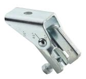
This code-compliant Structural Attachment is part of the nVent CADDY line of innovative rigid bracing system, designed to provide superior performance and meet the highest seismic load requirements. Its versatile design allows quick and easy installation directly to concrete, wood, bar joist or I-beam adapters and is compatible with 1" through 2" brace pipes. Its snap-off bolt makes inspection of seismic sway braces simple.
