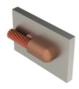
nVent ERICO Cadweld Cathodic Connections are the preferred method of exothermically welding cathodic protection anode leads to pipes (steel or cast iron), tanks, and other structures. Cathodic protection systems are designed to prevent galvanic corrosion along a pipeline or in various structures. nVent ERICO Cadweld Cathodic Connections use a special welding material alloy to minimize heat effect on the steel, which is especially important on thin wall and high stress pipes.
