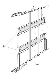
Bracket kit to make a 6 / 9 U Testadapter from 3 U Testadapters. Suitable for Testadapters with DIN 41612 connectors Type B, C, E and F.
