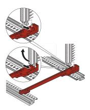
The the standard type guide rail with connector fixing allows the user to clip the DIN connectors directly onto the guide rails. Only applicable with Euroboards with the dimensions 100 x 160 mm and 100 x 220 mm. Suitable for RatiopacPRO/-AIR, PropacPRO, CompacPRO and EuropacPRO.
